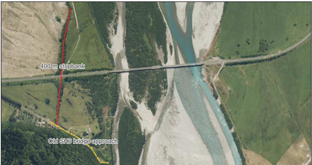
Figure 3-1 – The 400 m long true left stopbank immediately downstream of the old SH6 bridge.
