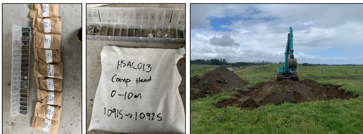
Figure 2 Photos of the sampling process. Left: Drill chip tray and 1m interval split samples for HSAC013. Centre: Composite samples made from the 1m interval split samples. Right: Bulk sampling test pit.
