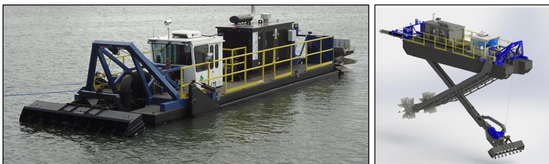
Figure 10: Example of a floating dredge (Source: Westland Mineral Sands Co. Ltd)
