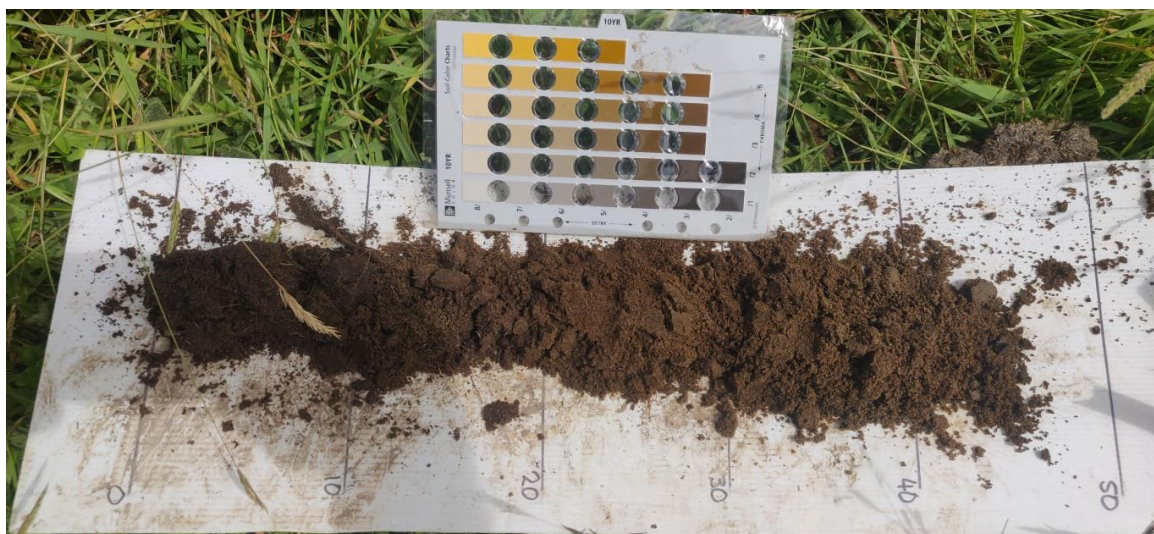
Plate 4. For reference, a dry non-hydric, upland soil taken approximately 15 m upgradient outside of the natural inland wetland in Plate 3.
