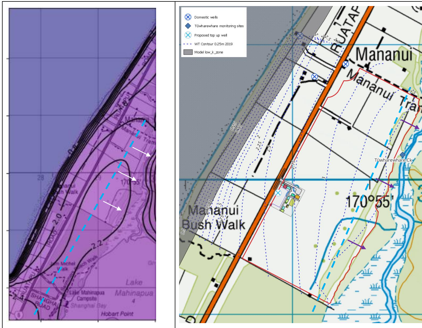
Figure 4-3: Modelled (left) and measurement-based (right) groundwater contours and flow divide
