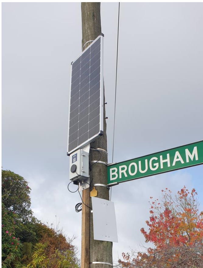
Figure 3: Photograph of a minimote mounted beneath a solar panel on a pole in Westport.
