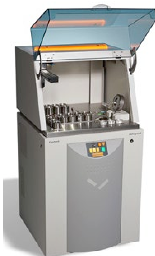
Figure A1.1 The PANalytical Epsilon 5 spectrometer.
