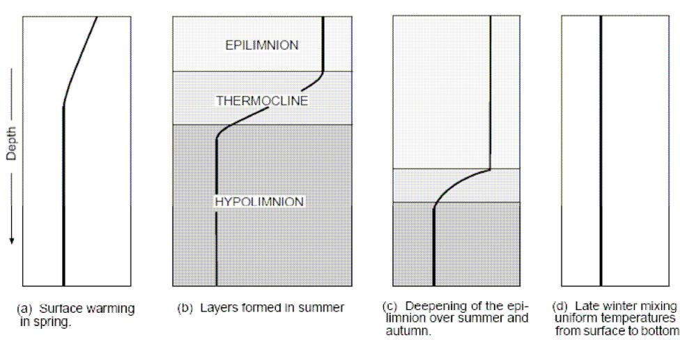
*Figure 5.13.2 The mixing cycle of the water of Lake Brunner. Each panel represents water temperature with depth in the lake for a particular season: (a) spring, (b) summer, (c) late summer/autumn, (d) late winter. Water temperature is represented by the thick black line in each panel with temperature increasing from left to right in each panel (courtesy of Kelly and Howard-Williams, 2003).*
