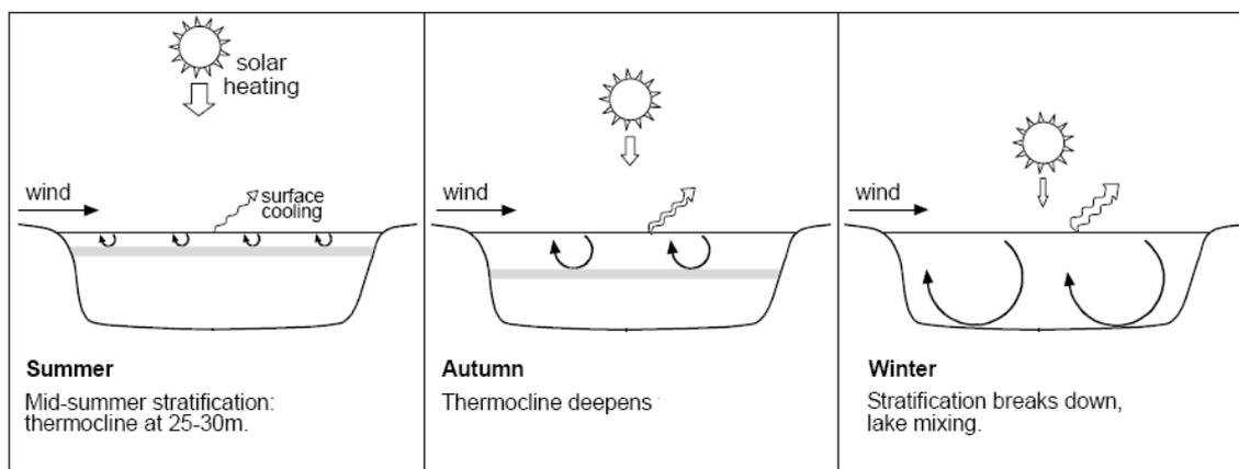
*Figure 5.13.1 Lake stratification and mixing is dependent on the interactions of the sun's energy and wind energy and on the net effect of heating and cooling. The sun tends to heat the lake and increase stratification, the wind tends to mix the lake and break down stratification (courtesy of Kelly and Howard-Williams, 2003).*
