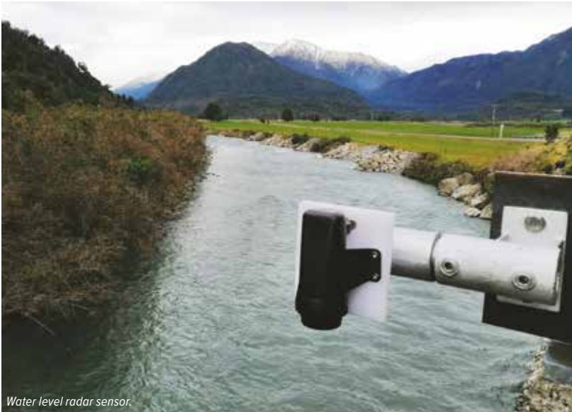
Water level radar sensor.
