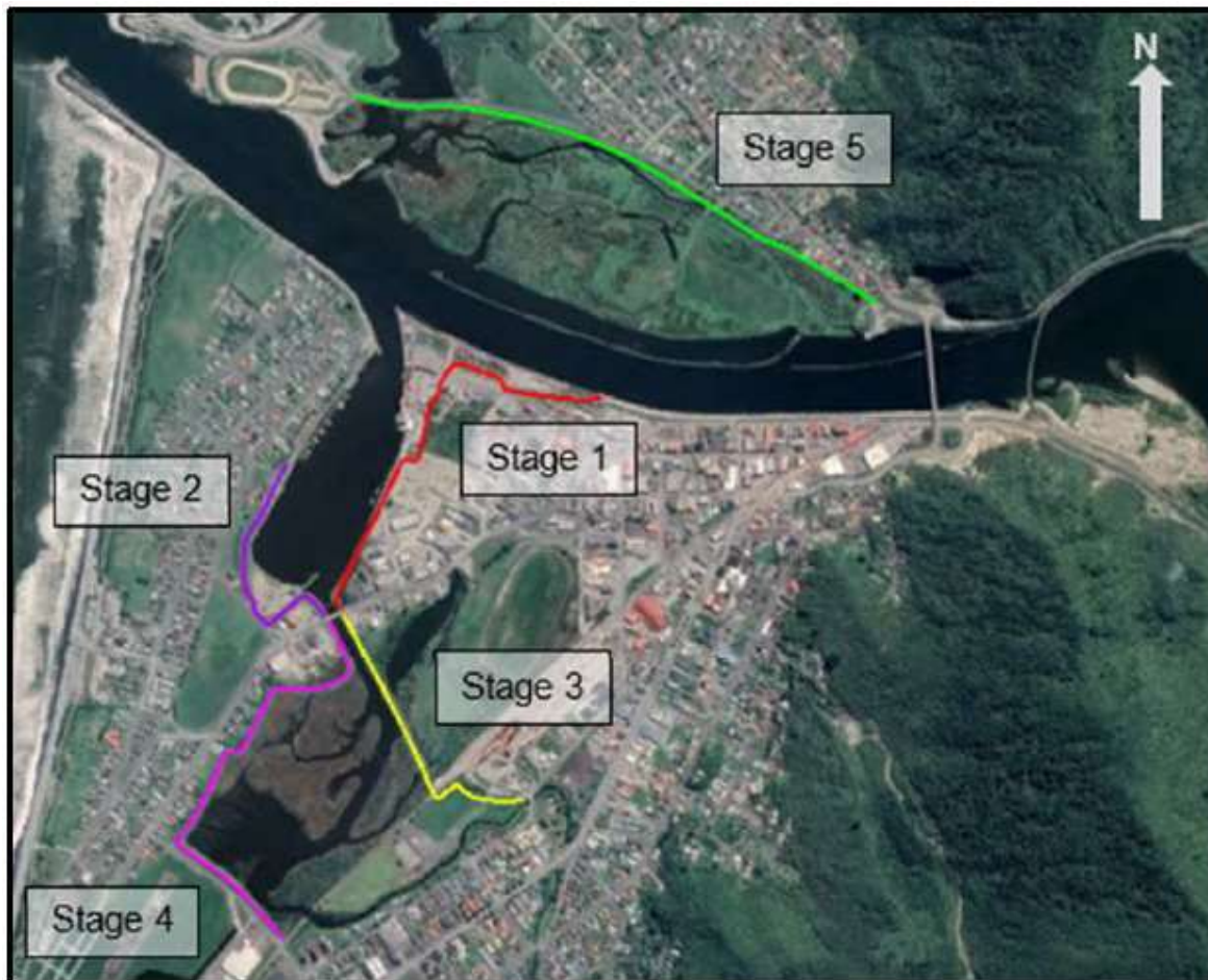
Figure 1: Greymouth Floodwall Upgrade Project Stages
