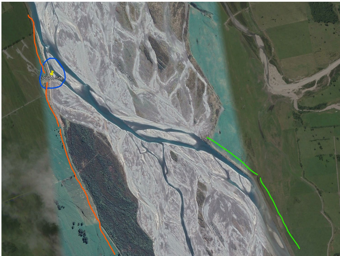
Figure 4: Green denotes Garland bank, orange denotes left bank stopbank, blue circle denotes job site.
